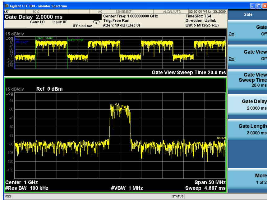
Figure 3-50 LTE TDD Uplink Monitor Spectrum Measurement Result - Gate View On
